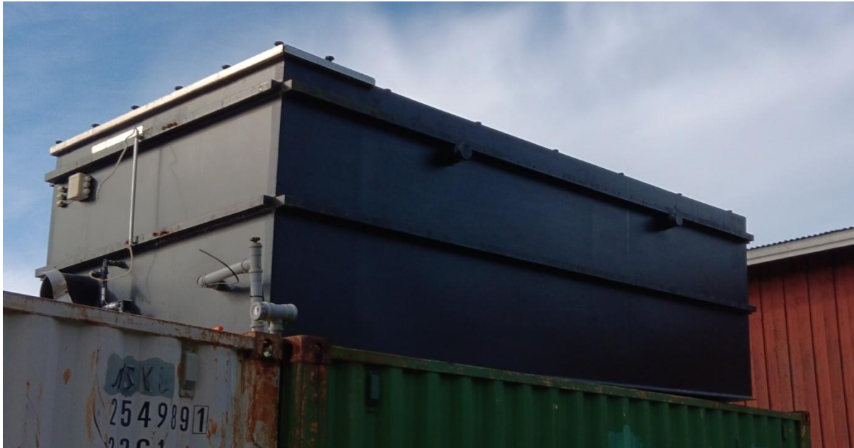
Figure 2. A steel tank which could be used for testing the leaching and dilution of organic materials.
